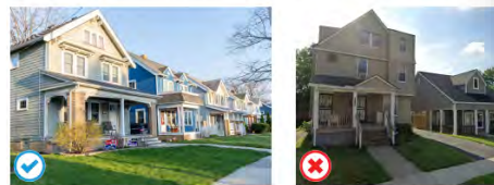
FIGURE 8 | NEIGHBORHOOD COMPATIBILITY This image shows how compatibility can allow differences among structures while still feeling cohesive on a neighborhood level. FIGURE 9 | INCOMPATIBILITY The dramatic differences in building and first floor height make the new (right) out of sync with neighborhood.
