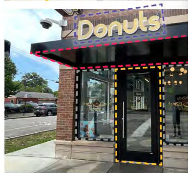
FIGURE 3 | COMPONENTS OF A STOREFRONT Well-designed storefronts with ample transparent windows, like the example shown, can help engage pedestrians and allow for more interaction between the building and the street.
