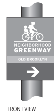
MOUNTED TO EXISTING UTILITY POLE SCALE: 3/8"=1'
