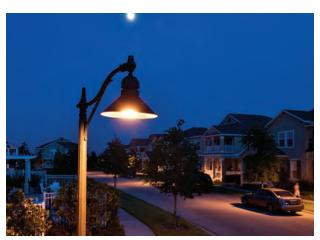
Dark sky compliant lighting shields the light source and focuses lighting downward to reduce light pollution.
