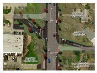
Plans for Royalton Road include the addition of two lanes, a five-foot wide sidewalk, a 10-foot wide shared use path, lighting, and green and grey stormwater infrastructure.
