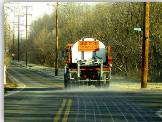
Figure 36: Salt brine solution being applied as pre-treatment City of Beavercreek, Ohio
